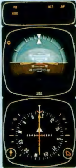
1. The aircraft is flying an OMNI airway in HDG mode on a heading of 80°.
