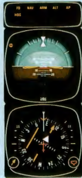
2. A waypoint has been established and the RNAV computer is in ENROUTE mode. A 112° course to the waypoint has been selected and NAV mode pushed "on". HDG and NAV/ARM modes are activated for automatic capture of the 112° course to the waypoint. The capture rate is now being computed based on closure rate. The airplane must be headed toward the selected course in order for NAV/CPLD to occur.
